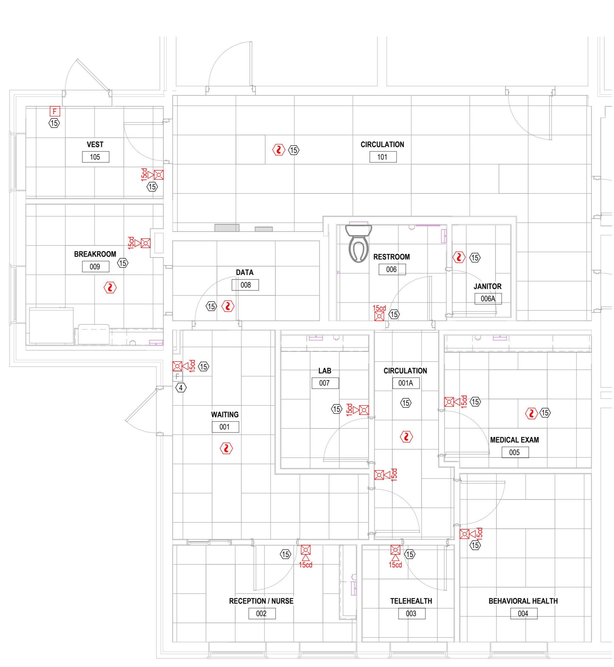
4 E1.0 ELECTRICAL FIRE ALARM PLAN 1/4" = 1'-0"
