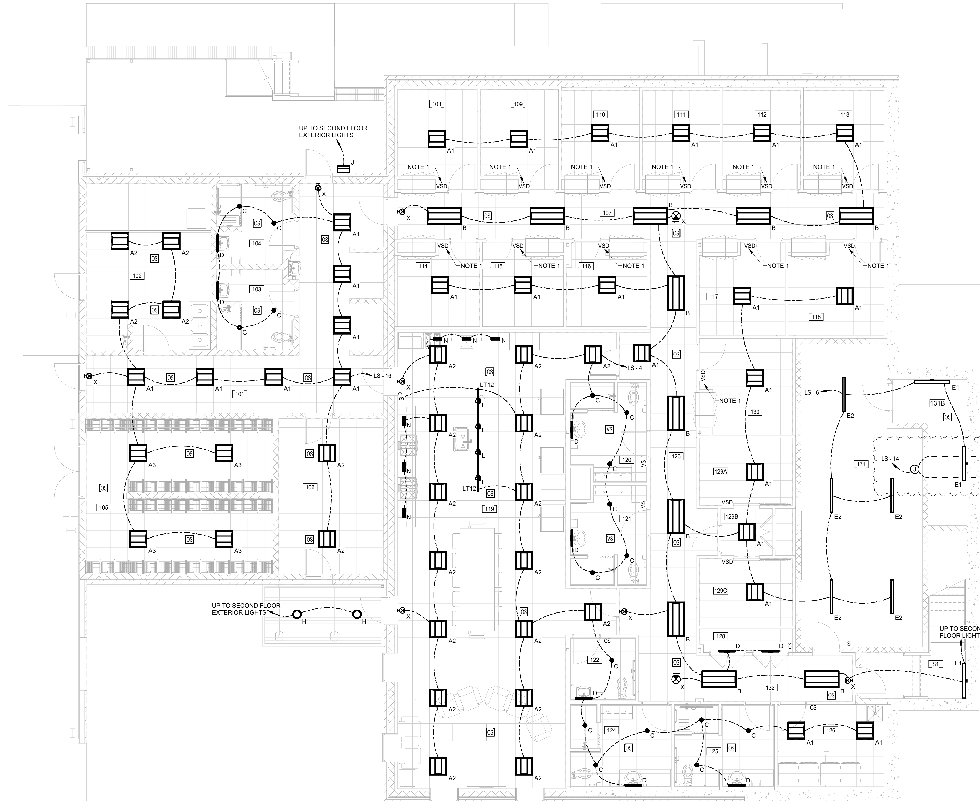
1 LIGHTING FIRST FLOOR PLAN (NOTE 2) E2.1 3/16" = 1'-0"
